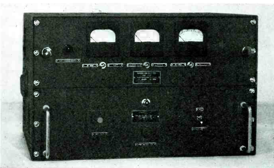
Fig. 16A, left. An electronic power supply unit to supply power for 24 large 2000 cycle inductance strain gages. Fig. 16, right. A power supply unit designed for use with type MRC-10 control unit to supply 5000 cycle power for carrier circuits and also all dc for amplifier elements
