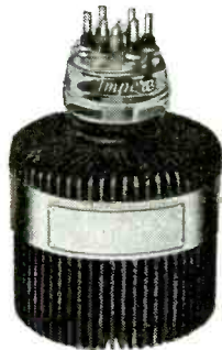
Amperex Type 235-R Transmitting Tube. Filament voltage, 14.5-15.0 volts. Filament current, 39.0 amperes. Amplification factor, 14.0. Grid to plate transconductance at 500 ma., 6500 micromhos. Direct interelectrode capacitance: grid to plate, 9.0 \mu\text{f} ; grid to filament, 10.0 \mu\text{f} ; plate to filament, 1.5 \mu\text{f} . List price, $125.00.
