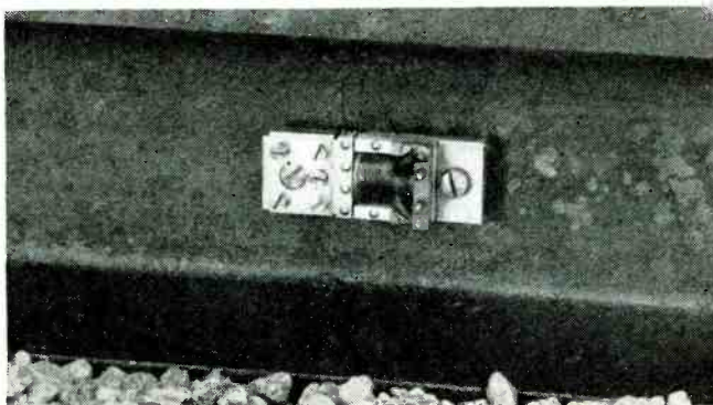
Fig. 1. Inductance type strain gage applied to a rail. As this must be screwed in place it is most used on large pieces. This gage measures strain at a point slightly off the surface thus permitting errors due to bending. This fault is not present in the type shown in Fig. 2, right
