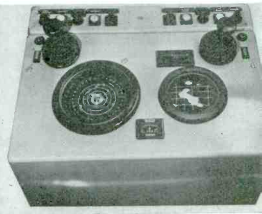
▼ Repeater for type SG radar. This can be located anywhere on the ship to give a PPI indication of objects surrounding the ship. The circles in the larger 'scope indicate distances. The smaller tube at the right presents an expanded view of a portion of the area scanned. Any portion can be chosen by turning one knob
