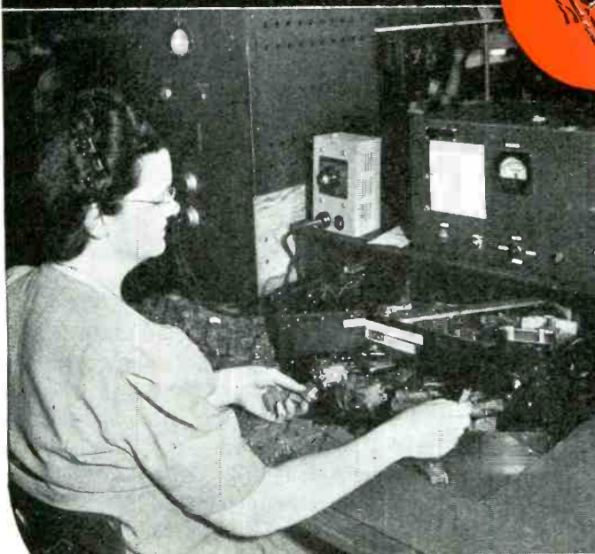
A view of the "merry-go-round" automatic checking equipment used for dielectric strength test.
