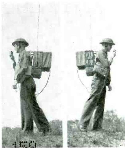
The equipment from both sides showing battery pack and antenna mounting
